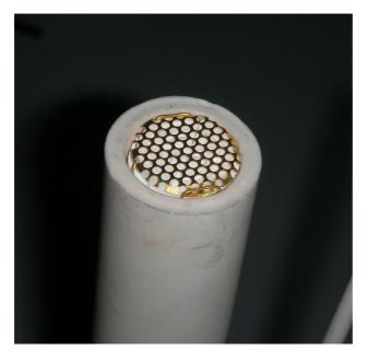
A one-inch sample holder mounted on the stand, with a detailed view of the optional laser machined contact grids on the gas diffusers.
