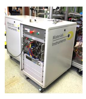
Materials Mates Italia (MMI) offers complete high-power solutions, from impedance spectroscopy to multichannel systems for stacks, including standard and customized cells. MMI also integrates in their systems a series of additional ancillary equipment to complete the test setup.
